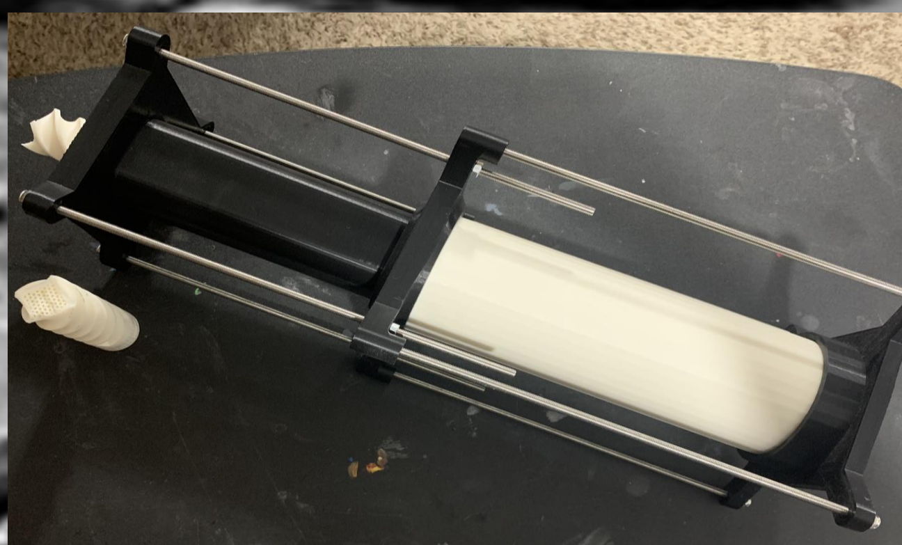
Figure 5 : Part Failure cause by initial testing.
