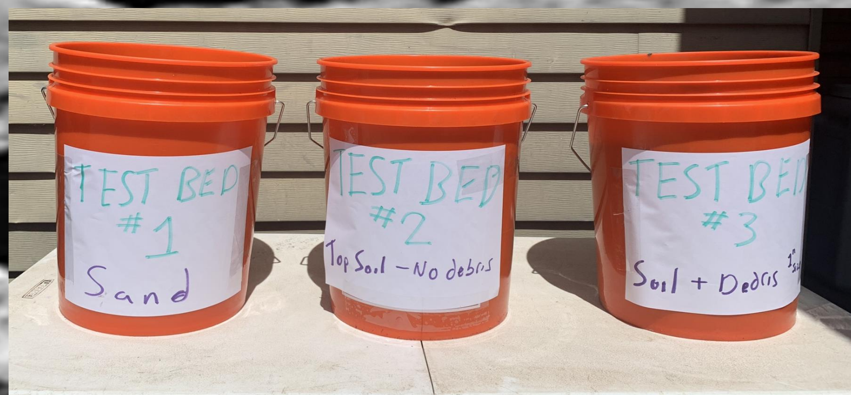
Figure 6: Initial Testing Beds, 3 different terrestrial soils
